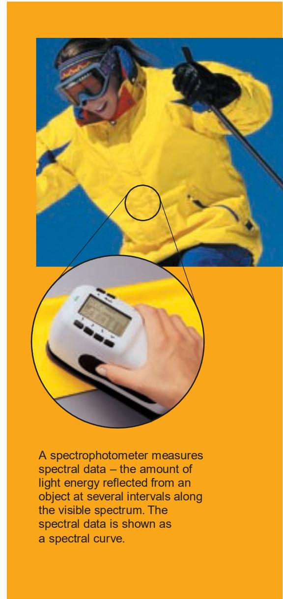
A spectrophotometer measures spectral data – the amount of light energy reflected from an object at several intervals along the visible spectrum. The spectral data is shown as a spectral curve.
